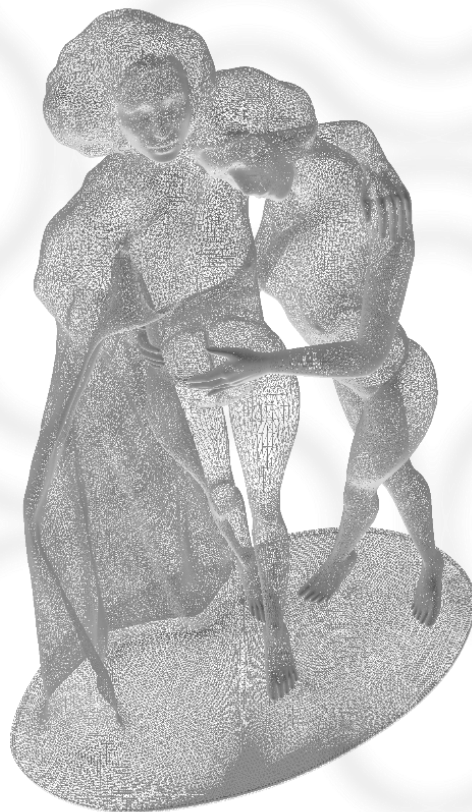
Figure 11. Elaborated 3D scanning, ready for a high-resolution 3D printing in wax, and afterwards lost wax manufacturing process in the foundry.
